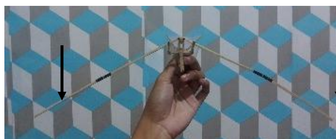
Fig. 10. Prototype's Flapping Motion on Downstroke
